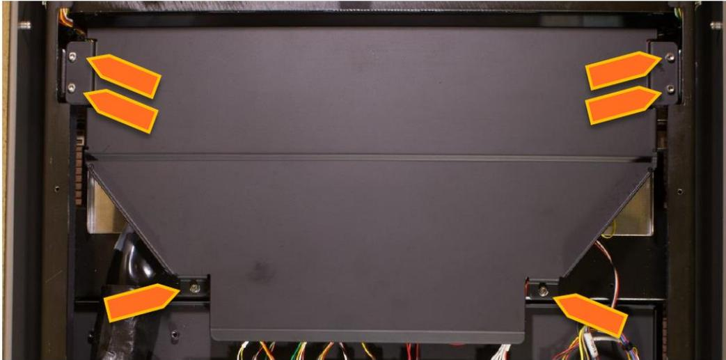
2.3 Remove 6 screws holding fiber bundle guide in position using 2.5mm hex key and remove the fiber guide.
