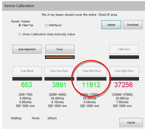
Figure 2.9 Proper Calibration
