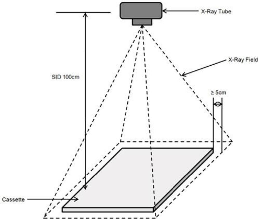
Figure 2.116 Calibration Geometry
