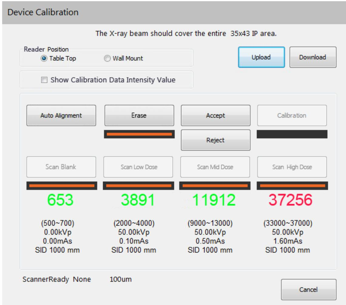
Figure 2.17 FireCR Flash IP Calibration
